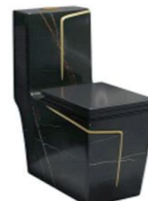
PL-086 Siphonic/Washdown one-piece toilet Size:680x355x780mm Siphonic/S-trap:250/300/400mm roughing-in Washdown/P-trap:180mm roughing-in
