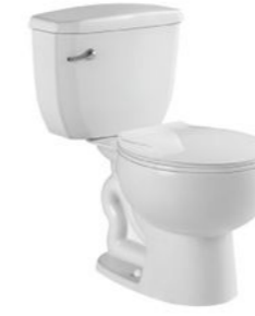
PL-6670 Washdown two-piece toilet Size:620x410x680mm S-trap 250mm roughing-in P-trap 180mm roughing-in
