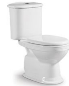
PL-6618 Washdown two-piece toilet Size: 660x400x770mm P-trap 180mm roughing-in S-trap 250mm roughing-in
