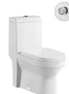
PL-3858 Washdown&Siphonic one-piece toilet Size:710x365x800mm S-trap 250/300mm roughing-in P-trap 180mm roughing-in
