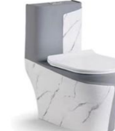
PL-3899-9 Siphonic/Washdown one-piece toilet Size: 690x390x740mm Siphonic/S-trap: 250/300/400mm roughing-in Washdown/P-trap: 180mm roughing-in
