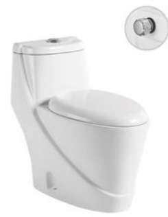
PL-3893 Washdown one-piece toilet Size:740x360x740mm S-trap 250mm roughing-in P-trap 180mm roughing-in
