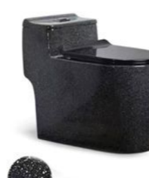
PL-3047-3 Siphonic/Washdown one-piece toilet Size: 700x365x600mm Siphonic/S-trap: 250/300/400mm roughing-in Washdown/P-trap: 180mm roughing-in
