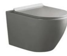
PL-7774-3 Rimless wall hung toilet Size:535x365x360mm P-trap180mm roughing-in
