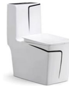
PL-3890-B Siphonic/Washdown one-piece toilet Size: 685x355x775mm Siphonic/S-trap: 250/300/400mm roughing-in Washdown/P-trap: 180mm roughing-in
