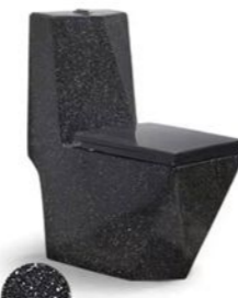
PL-3814-3 Siphonic/Washdown one-piece toilet Size: 700x370x835mm Siphonic/S-trap: 250/300/400mm roughing-in Washdown/P-trap: 180mm roughing-in
