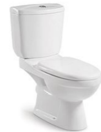
PL-6614 Washdown two-piece toilet Size: 700x380x740mm P-trap 180mm roughing-in S-trap 100/250mm roughing-in
