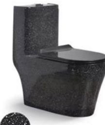
PL-3899-3 Siphonic/Washdown one-piece toilet Size: 690x390x740mm Siphonic/S-trap: 250/300/400mm roughing-in Washdown/P-trap: 180mm roughing-in
