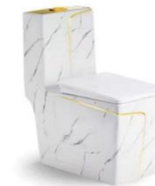
PL-3890-5 Siphonic/Washdown one-piece toilet Size: 685x355x775mm Siphonic/S-trap: 250/300/400mm roughing-in Washdown/P-trap: 180mm roughing-in
