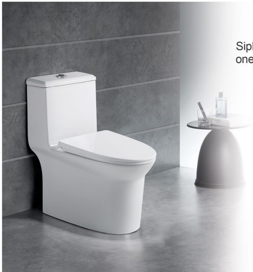
PL-3886 Washdown one-piece toilet Size:700x385x760mm S-trap 250mm roughing-in P-trap 180mm roughing-in
