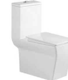
PL-3863 Washdown one-piece toilet Size:700x380x820mm S-trap 250mm roughing-in P-trap 180mm roughing-in
