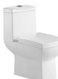
PL-3830 Siphonic one-piece toilet Size:660x350x770mm S-trap 220/250/300mm roughing-in P-trap 180mm roughing-in
