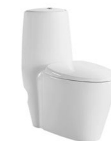
PL-3833 Washdown one-piece toilet Size:700x380x780mm S-trap 250mm roughing-in P-trap 180mm roughing-in
