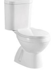
PL-6105 Washdown two-piece toilet Size:640x375x795mm S-trap 250mm roughing-in P-trap 180mm roughing-in
