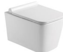
PL-7797 Washdown wall-hung toilet Size:540x365x350mm P-trap 180mm roughing-in
