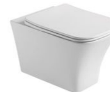
PL-7800 Rimless wall hung toilet Size:520x360x370mm P-trap 180mm roughing-in
