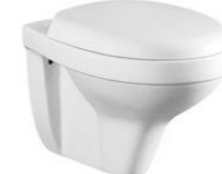
PL-7711 Washdown wall-hung toilet Size:560x340x380mm P-trap 180mm roughing-in
