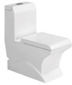
PL-3881 Washdown one-piece toilet Size:755x365x770mm S-trap 250mm roughing-in P-trap 180mm roughing-in
