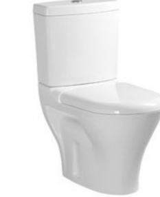
PL-6604 Washdown two-piece toilet Size:670x375x820mm S-trap 250mm roughing-in P-trap 180mm roughing-in
