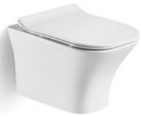
PL-7117 Rimless wall hung toilet Size: 490x340x360mm P-trap 180mm roughing-in
