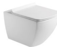
PL-7799 Rimless wall hung toilet Size:520x360x370mm P-trap 180mm roughing-in
